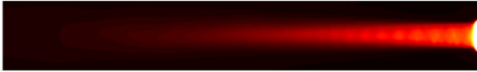
Figure 8: Case 1 Measurement – Plume Apparent Contrast Radiant Intensity = 0.51\text{Wsr}^{-1}
